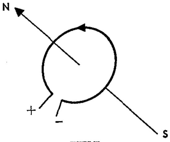
FIGURE XL Magnetic Field Around Loop.
