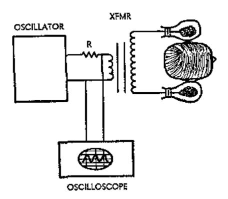
FIGURE VI Measuring resonance.
